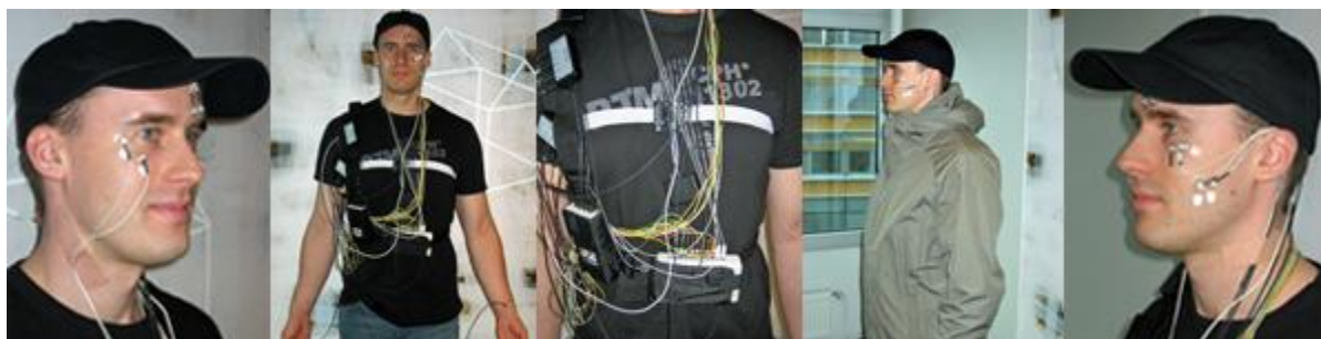
Figure 1. A mobile physiological data acquisition system (Varioport-B) used to study psychophysiological responses during mobile gaming.
